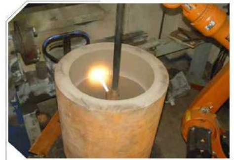
GUN EXTENSION FOR INTERNAL COATING
