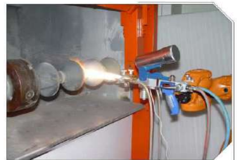
ANTI-WEAR COATING ON TEXTILE INDUSTRY PARTS
