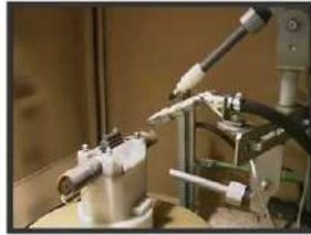
CNC 2 AXES CERAMIC/GLASS BEAD PEENING MACHINE
