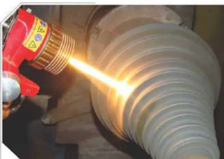
HARD COATING ON TEXTILE INDUSTRY PARTS
