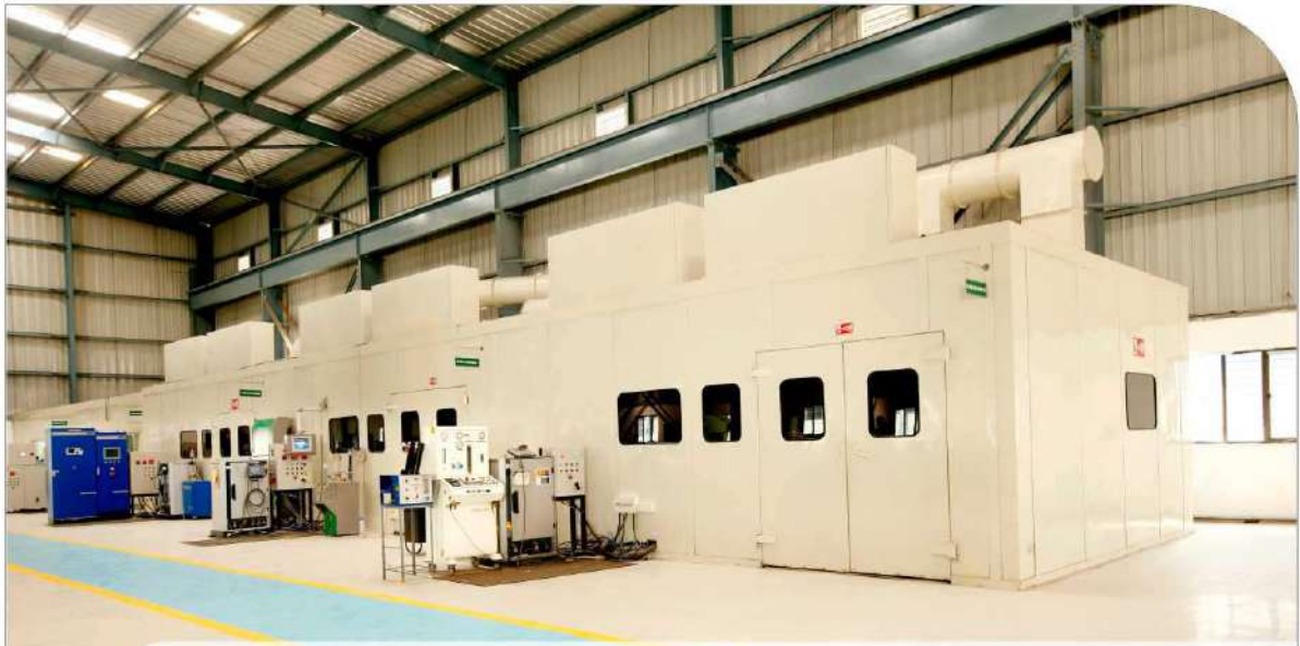
5 ROOMS SETUP FOR DETONATION GUN, HVOF & PLASMA
