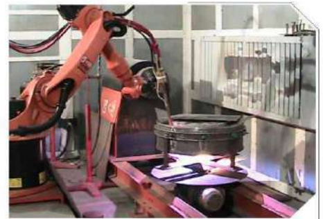
HIGH TEMPERATURE RESISTANCE COATING ON GAS TURBINE PARTS
