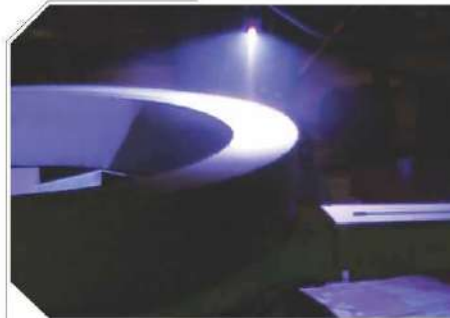
ANTI - CORROSION COATING ON WIND MILL PARTS
