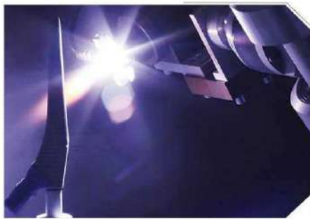
ORTHOPEDIC IMPLANTS COATING BY PLASMA
