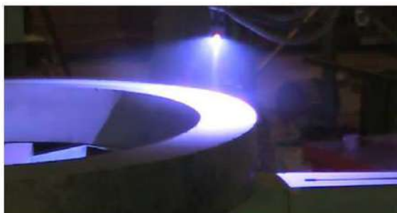
ARCJET ® -99ED TWIN WIRE ARC-SPRAY SYSTEM
