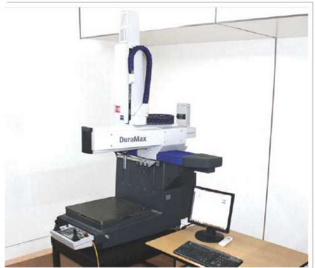
QUALITY CONTROL USING MODERN CMM
