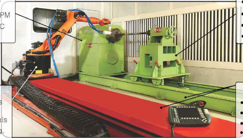
6 AXES ROBOT WITH 7 TH AXIS LINER TRACK
