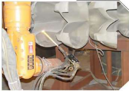
ANTI-WEAR COATING ON HYDRO TURBINE COMPONENTS
